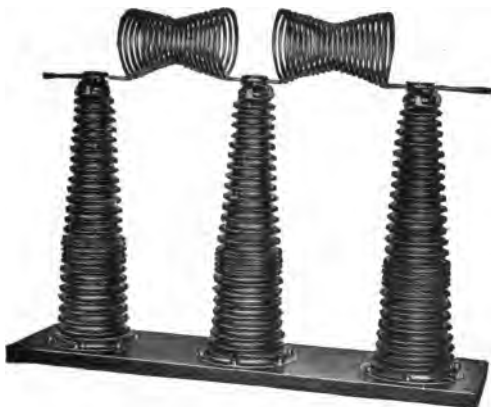
FIG. 231. Hour glass choke coils for 110,000-volt lines. These coils choke back the steep-front and high-frequency waves due to lightning discharges in the vicinity of the line. The General Electric Co.
